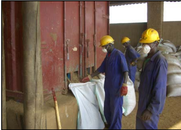
Medium and Large grade Vermiculite being bagged from screen separator
