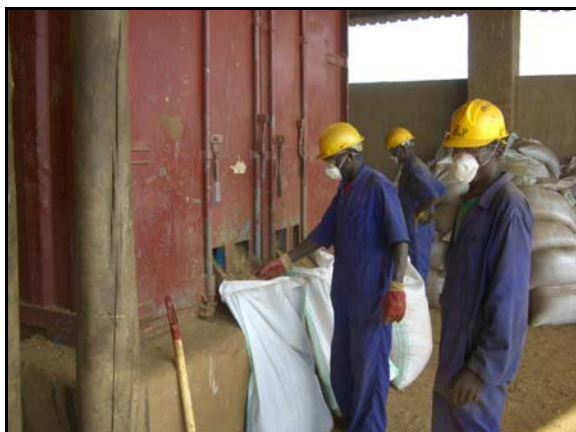
Medium and Large grade Vermiculite being bagged from screen separator
